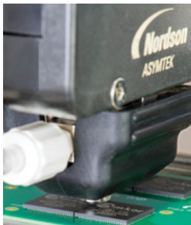
Ultra-precise placement of <200 \mu m fluid stream widths into narrow gaps
